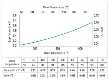
\*MinWool-1200 Pipe & Tank Insulation as tested in accordance with ASTM C518.
